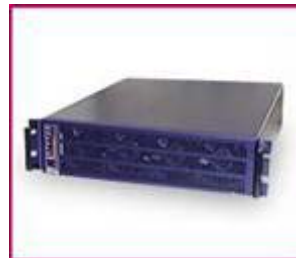
Hamamatsu Metrix Co., Ltd. developed a multi-particle high-speed super parallel calculating device, the GRAPE6B
