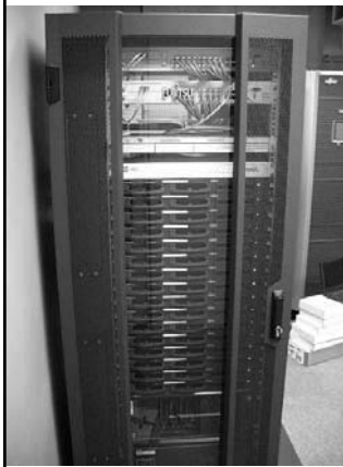
Fujitsu PRIMERGY—L200 16 nodes, 32CPU Pentium III 1.2 GHz Hi-per BLAST System Installed in Yasunaga Lab., Genome Information Research Center
