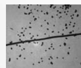
Powder RFID chips next to the human hair
